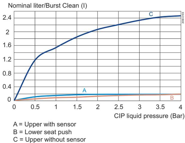
**Figure 5. Unique Mixproof valve / Unique Mixproof CP-3 valve
