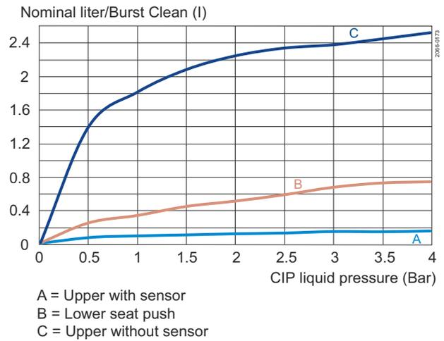
**Figure 8. Unique Mixproof valve / Unique Mixproof CP-3 valve with lower flush**
