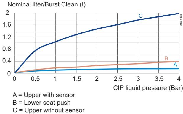
**Figure 3. Unique Mixproof valve / Unique Mixproof CP-3 valve
