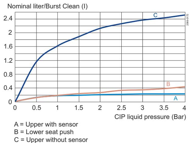
**Figure 6. Unique Mixproof valve / Unique Mixproof CP-3 valve with lower flush
