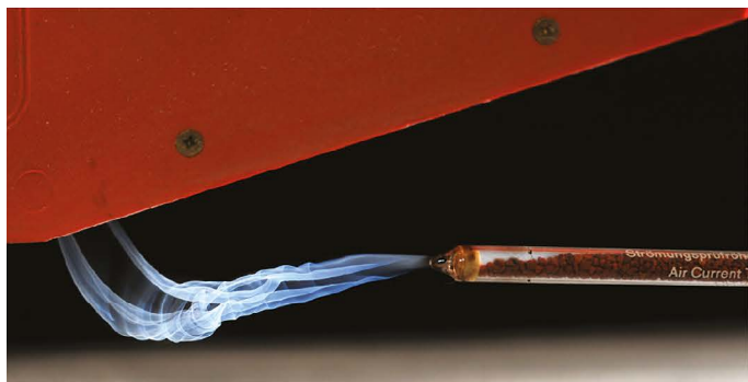
Figure 15a: Shows a smoke tube.
